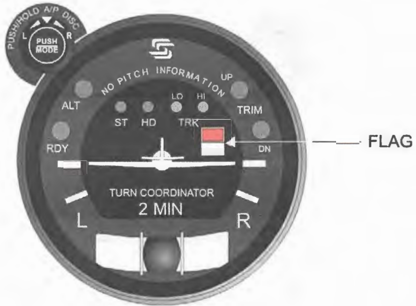
Fig. 2-12. AP Display, Low Voltage Flag (System Thirty)
