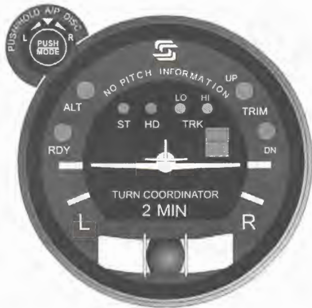
Fig. 2-9. AP Display, All Lamps Extinguished (System Thirty)
