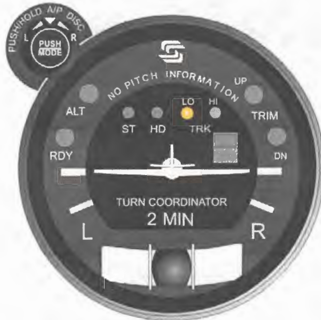
Fig. 3-3. AP Display, LO TRK Mode Engaged
