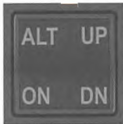
Fig. 2-16. ALT HOLD ON/OFF Switch Display, ALT ON Lamp Extinguished (System Thirty ALT)
