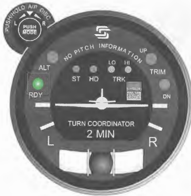
Fig. 2-10. AP Display, RDY for Operation (System Thirty)
