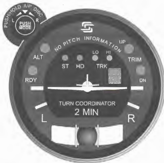
Fig. 2-11. AP Display, Turn Coordinator Failure (System Thirty)
