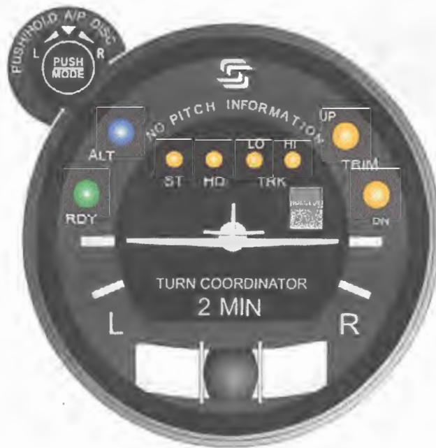
Fig. 2-6. AP Display, RDY, ALT, ST, HD, LO TRK, HI TRK, TRIM UP, TRIM DN Lamps Illuminated at Power-Up (System Thirty)
